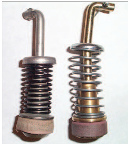
Compare all the pump pistons, reject those obviously shorter than the others.
