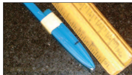
Plastic straw, .2" diameter, folded and taped. Mark 3/4" + from bottom of the fold. Filled through the short end, the volume below the mark holds very close to the .3cc. spec. Instant calibrated vial.
